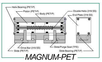
The PET unit is de-ionized (D.I.) water tolerant for use in hard disk and epitaxial fabrication. All materials used in the "PET" version of the MAGNUM comply with FDA requirements for food handling.
